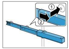
2. Place the telescopic rail on the rear pin ① and push the locking mechanism back ②.
