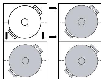
The cookware is detected and the previously selected power level flashes on the display for the new cooking zone.
