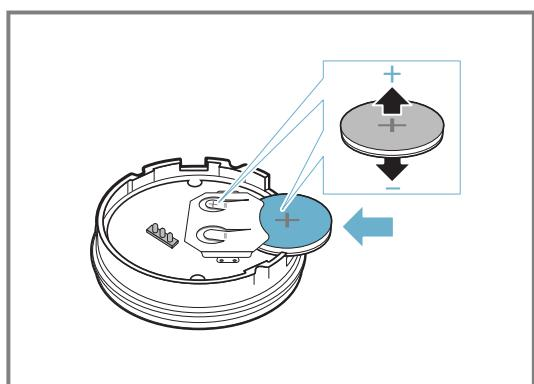
**Note:** Do not use any metal objects to remove the battery. Do not touch the battery connection points.
