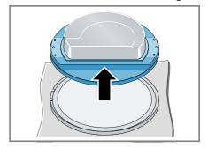
4. Turn the door ring by 180 ① and insert the door into the door ring ②
