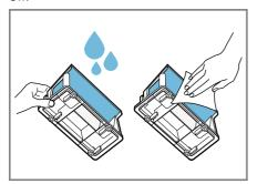
You can remove heavy soiling carefully with a soft brush. Ensure that you thoroughly dry off the filter. If the filter is damp, this may increase the drying time and affect the drying result.
