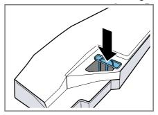
5. Insert the condensation container. → "Inserting the condensation container", Page 39
