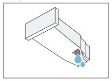
Check the condensation container filter → Page 52 regularly and clean the filter if it is dirty. Make sure that you insert the condensation container before operating the appliance.
