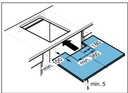
8. Observe the clearance between the intermediate floor and the worktop.
