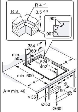
5. Ensure that the angle of the cut surface to the worktop is  $90^{\circ}$ .
