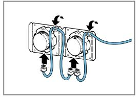
The two connectors on the control knob are identical.
