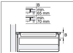
**4.** Mark the unit cut-out in accordance with the installation diagram.
