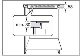
**3.** Maintain the minimum clearance from the upper edge of the worktop to the upper edge of a drawer installed below it.
