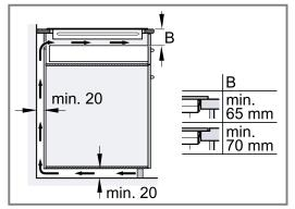
**3.** If there is no minimum clearance at the rear of the unit, make a unit cut-out in the bottom of the unit.
