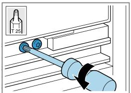
3. Adjust the door and tighten both screws.
