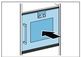
**4.** Centre the appliance. There must be an air gap of at least 2 mm between the appliance and the adjacent unit fronts.
