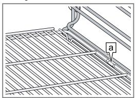
2. Ensure that the safety bar a on the wire rack is located at the rear and is facing upwards.
