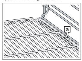
The catch tappets are located on the left and right of the wire rack at the centre on the outside.
