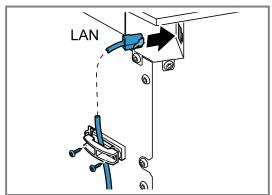
3. Connect the LAN cable to a network connection.
