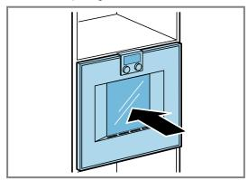
4. Centre the appliance. There must be an air gap of at least 2 mm between the appliance and the adjacent unit fronts.
