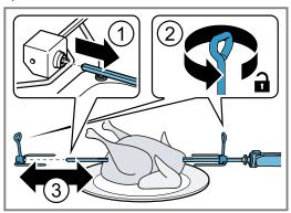
**7.** Press the button on the handle to remove it.
