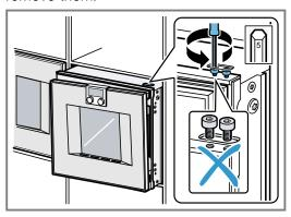
3. Adjust the appliance door using the side screw; to do this, open the appliance door and then close it again if necessary.
