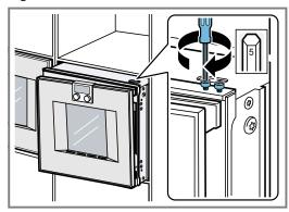
6. Slide the appliance into the built-in recess.
