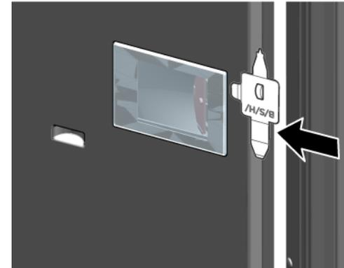
2. Pull LED spot light cover inwards and simultaneously push forwards.
