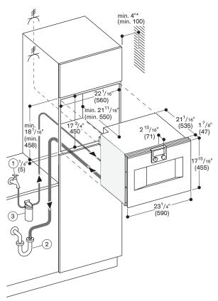
\* 8" (200) minimum when installed with handle.
