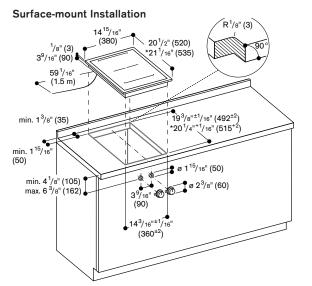
\* with appliance cover or adjustment strip. See separate planning notes on page 93. \*\*  $3\%_{16}"(90)$  in the area of the wire connection (rear, right).
