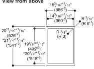
\* with appliance cover or adjustment strip (observe front and rear asymmetrical assembly. See separate notes "assembly with appliance cover/adjustment strip" on page 93).
