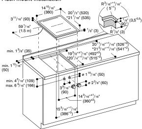
$^*$  with appliance cover or adjustment strip. See separate planning notes on page 93. \*\* 31¼ e<sup>i</sup>(93) in the area of the wire connection (rear, right).
