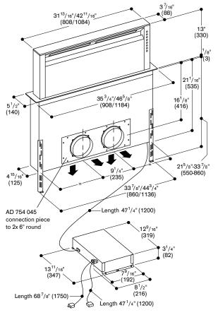
Duct connection 2 x ø 6" front/back Round duct connection piece with AD 754 045
