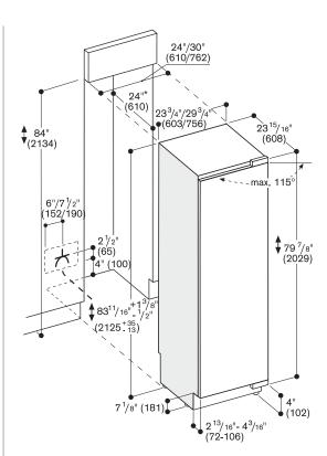
The door face dimensions are designed for a maximum gap of 1/8" (3 mm).
