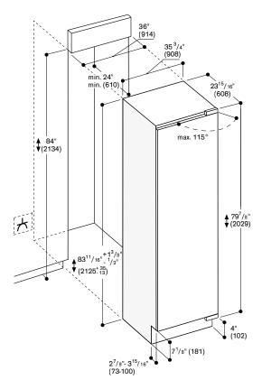
The door face dimensions are designed for a maximum gap of  $\mbox{\em 1/6}"$  (3 mm). See more details on page 247.
