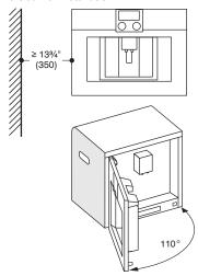
If using the 92° door hinge restrictor (spare part no. 00636455), the minimum distance from the wall is only 4" (100).
