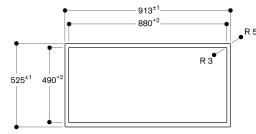
measurements in mm
