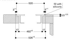
When installing with appliance cover or filler strip, pay attention to the deeper cut-out and the front and rear groove width.
