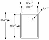
A: When installing with appliance cover, take the deeper cut-out into consideration (observe separate planning notes)
