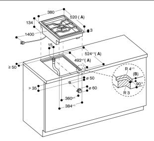
A: When installing with appliance cover consider the deeper cut-out (observe separate planning notes)
