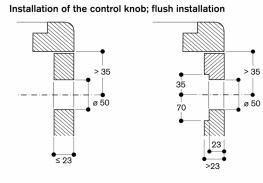
measurements in mm
