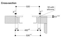
When installing with appliance cover or filler strip, pay attention to the deeper cut-out and the front and rear groove width.
