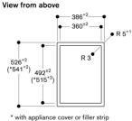
with appliance cover or filler strip (observe the front and rear asymmetrical support, see separate notes "Installation with appliance cover/filler strip").
