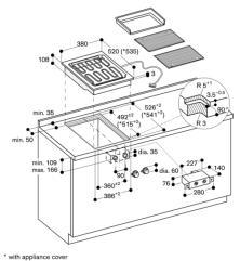
\* with appliance cover measurements in mm
