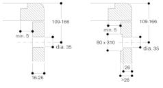
Installation with appliance cover/spacer batten; installation standing proud of surrounding surfaces
