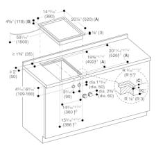
A: When installing with appliance cover, take the deeper cut-out into consideration (observe separate planning notes) B: 5¼° (133 mm) in the area of the cable clamp (left, on the rear side) C: ⅓° (3.5°°) measurements in inches (mm)
