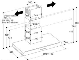
Air extraction: Recirculation: AD 280/281 012 = 650–1,020 mm AD 280/281 112 = 760–1020 mm AD 280/281 022 = 1020–1410 mmAD 280/281 122 = 1020–1410 mm
