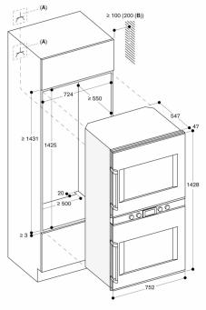
A: Electrical connection B: 200 mm in conjunction with BA 018 Measurements in mm
