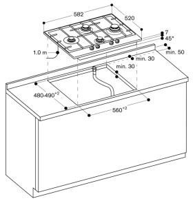
\* 56 mm in the area of the gas connection at the back right
