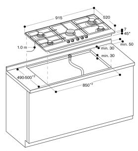
\* 61 mm in the area of the gas connection at the back right
