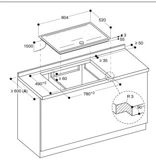
A: Please check the installation manual if the worktop depth is less than 600 mm.
