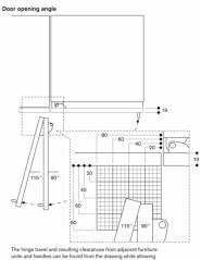
The mige travel and resulting clearances from adjacent furniture units and handles can be found from the drawing while allowing for the thickness of the front panel. In the drawing, a furniture un front panel thickness of 19 mm was assumed.
