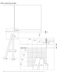
units and handles can be found from the drawing while allowing for the thickness of the front panel. In the drawing, a furniture unit front panel thickness of 19 mm was assumed.
