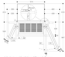
וא In the drawing, a unit front thickness of 19 mm and a Gaggenau unit handle of 49 mm were taken as a basis.
