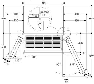
In the drawing, a unit front thickness of 19 mm and a Gaggenau unit handle of 49 mm were taken as a basis.
