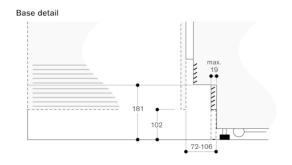
Based on the standard height of the appliance, the height of the plinth is 102 mm. Maximum thickness of the plinth is 19 mm.
