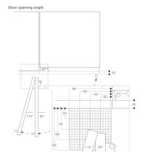
The hinge travel and resulting clearances from adjacent furniture units and handles can be found from the drawing while allowing for the thickness of the front panel. In the drawing, a furniture uniform problem of 19 mm ups sesumed.
