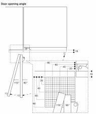
The hinge travel and resulting clearances from adjacent furniture units and handles can be found from the drawing while allowing for the thickness of the front panel. In the drawing, a furniture uni front panel thickness of 19 mm was assumed.
