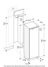
Based on the standard appliance height, the height of the plinth is 102 mm. Maximum plinth thickness 19 mm.
