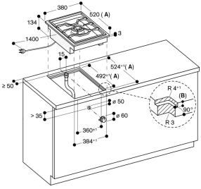
**A:** When installing with appliance cover consider the deeper cut-out (observe separate planning notes)
