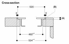
A:  $3.5^{\circ.5}$  6.5\*0.5in combinations with frameless induction hobs B: Fill with silicone
