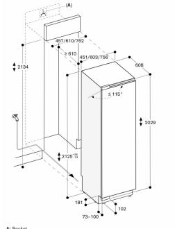
A: Socket Maximum door panel dimensions are based on a clearance of 3 mm
