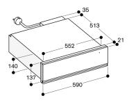
measurements in mm
