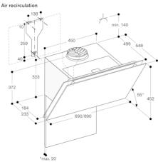
\* Note the maximum thickness of the back panel.
