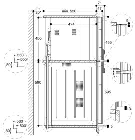
\* Only required if the water hoses for the BS steam oven cannot be accommodated in the corner recesses of the appliances.
