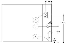
(4) electric terminal box(5) cold-water connection(6) water outlet
