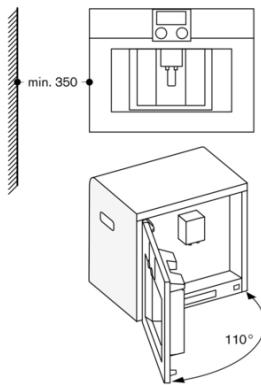
If using the 92° door hinge restrictor (spare part no. 00636455), the minimum distance from the wall is only 100 mm.
