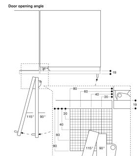
The hinge travel and resulting clearances from adjacent furniture units and handles can be found from the drawing while allowing for the thickness of the front panel. In the drawing, a furniture unit front panel thickness of 19 mm was assumed.
