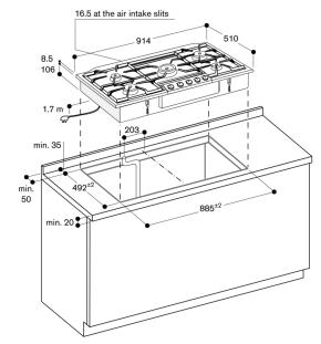
Minimum distance from the appliance cut-out to the side wall 300 mm.
