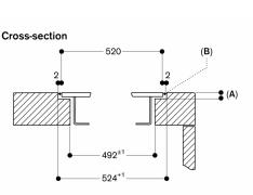
A: 3.5<sup>-05</sup> 6.5<sup>+05</sup>in combinations with frameless induction hobs B: Fill with silicone
