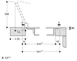
measurements in mm
