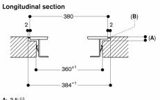
A: 3.5<sup>-05</sup> 6.5<sup>+05</sup>in combinations with frameless induction hobs B: Fill with silicone
