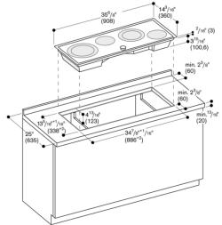
Immersion depth in the area of the electric connection casing  $4^{13}/16^{\prime\prime}$  (123)
