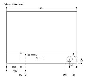
A:LAN connection B:Electric terminal box C:Water outlet D:Cold water inlet
