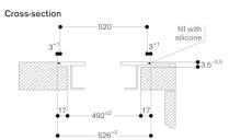
When installing with appliance cover or filler strip, pay attention to the deeper cut-out and the front and rear groove width.
