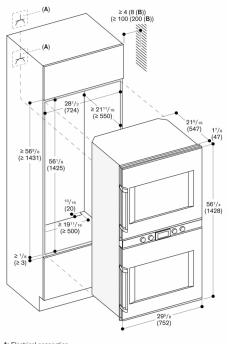
A: Electrical connection B: 8" (200 mm) in conjunction with BA 018 Measurements in inches (mm)
