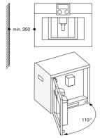
If using the  $92^{\circ}$  door hinge restrictor (spare part no. 00636455), the minimum distance from the wall is only 100 mm.
