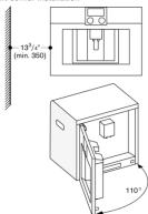
If using the 92° door-hinge restrictor (spare part no. 00636455), the minimum distance to the wall is only  $3^{15}/\mbox{\scriptsize 16}^{\circ}$  (100 mm).
